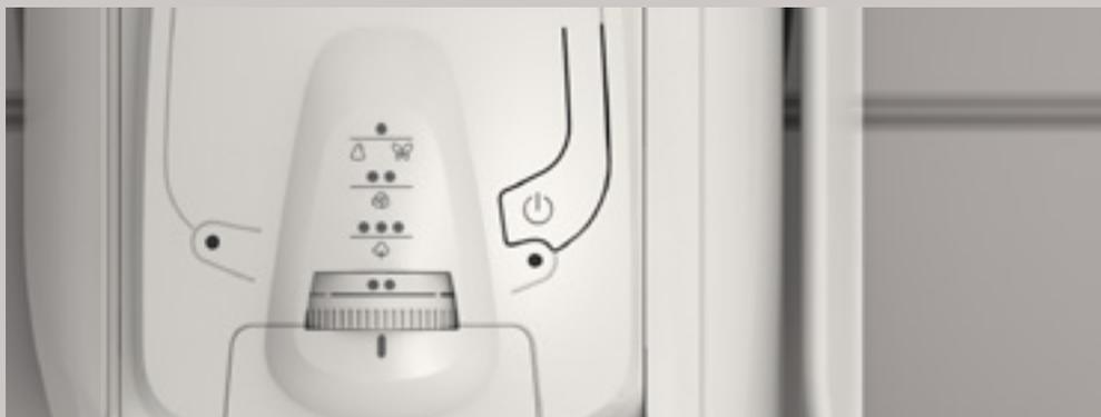
With the press still open, press the digital pressure on/off button. The green and red lights will illuminate to indicate that the press is on and warming up. Turn the temperature regulator up to the desired level. When the right temperature is reached, the red light will switch off. To switch off the press, press lightly on the digital pressure switch again.
