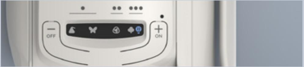
Slightly press the ON button with the press open.
